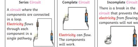
There is a break in the circuit that prevents the electricity from flowing. The components will not work.
